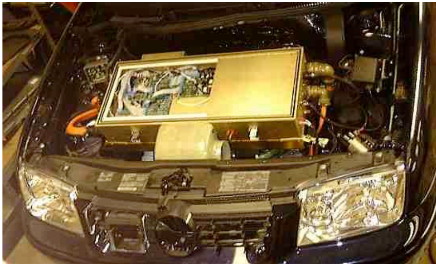
Figure 3. Electric Drive System Installed
